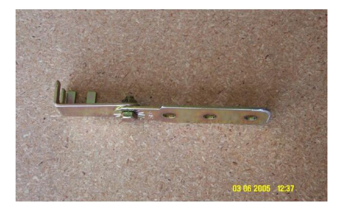
Fabricate a bracket for the control switches. My bracket is constructed from .06 aluminum and it also holds a handheld 2-way radio to the right. The Audiovox directions include the dimensions for the slot in the bracket. The slot is for the wires coming off the back of the switch unit.
