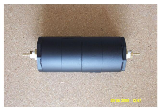
My friend constructed his vacuum canister from a 5" length of 2" ABS and two 2" ABS end caps. He drilled the ends, threaded and cemented the brass barb fittings into place. This unit is lighter than the PVC and is already black.
