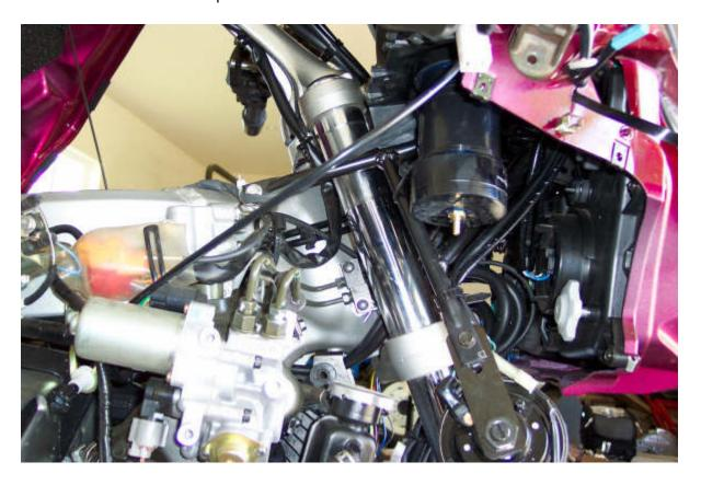
Cut a short piece of vacuum hose and connect the check valve to the vacuum canister. Make sure the check valve is in the right direction (the engine pulls a vacuum on the canister).
