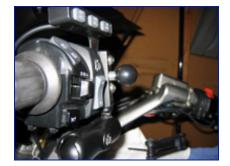
Routing the wiring for it was not too tough just take time to give enough slack so it gives when turning the handlebars from side to side.
