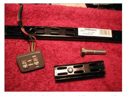
I mounted my control pad on the handle bar using the unused 10mm mirror mount. I made a very solid bracket using two 4" lengths of adjustable bookshelf support. It's even black and I won't have to paint it!
