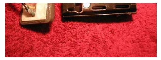
Weatherproof the control pad by taking it apart and removing the membrane switches from the housing. Smear some silicone adhesive around the holes in the housing and replace the membrane. Snap the control pad back together then smear some more silicone around the seam on the back and gob a liberal amount around the wires where they come out the back. Looks waterproof to me.
