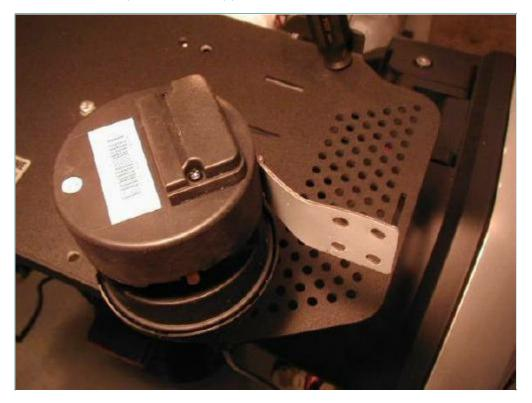
By holding the unit in position under the right side cover and putting the bracket between the tool tray (remove the 10mm mounting bolt) and the frame, you can decide where and how much the bracket should be bent to facilitate an installation which will not interfere with the side cover when it is reinstalled.
