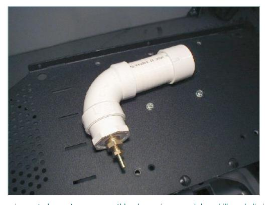
To make the cruise control operate more smoothly when going up and down hills and eliminate surging, it is desirable to add an extension vacuum canister to increase the vacuum capacity of the unit. The actual configuration here is pretty subjective, but this particular setup will work and is shaped to fit in the small space left around the servo.
