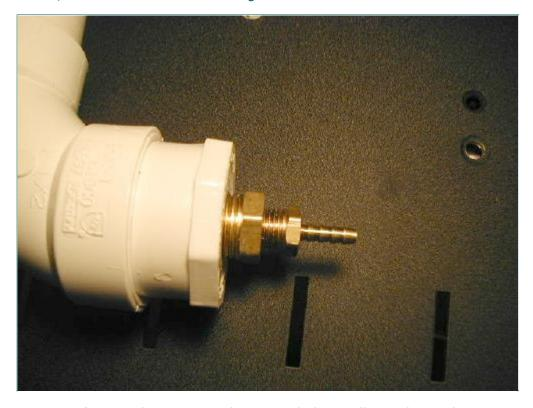
Sand all PVC mating surfaces with coarse sandpaper and glue it all together with a coating of adhesive. After assembling each glued joint, give it a 1/4 turn twist to make a more positive seal. Use the Teflon tape to make a couple rounds of each brass fitting thread and wrench the fittings together until they are snug.
