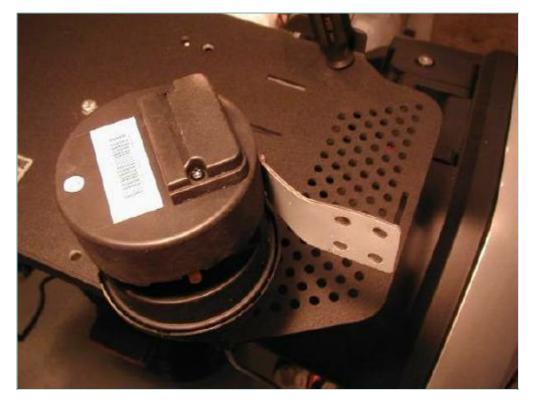
On the end opposite the long servo cable, unscrew the small plastic cover.
