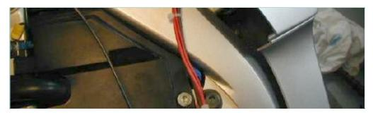
Knowing that, route the protected harness forward from the servo, behind the frame, and up into the engine compartment under the gas tank. I looped the extra length around the top of the engine.
