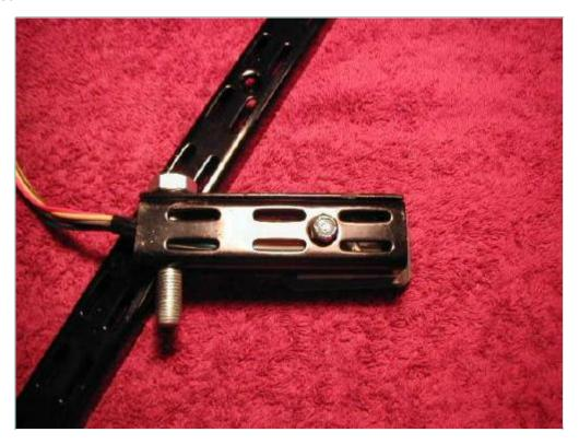
Here the control pad is mounted to the bracket with the included 3M tape and the wires are routed through the bracket and out the end. I put some heat shrink tube on the wires and the machine screw to prevent chafing.
