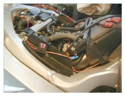
The Red wire goes to Switched 12volt power for the Control Pad electronics and is fused, so locate it where it is accessable.
