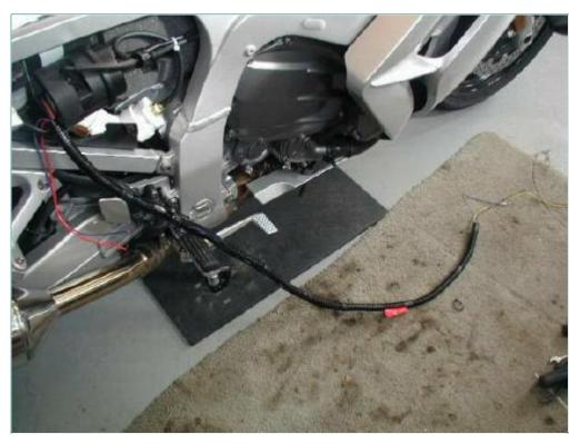
Find the Black and Gray wires that are harnessed together. These won't be used so double them back along the harness, tape them to the other wires in a couple spots, then stuff the wires into the convoluted harness protector from the kit.
