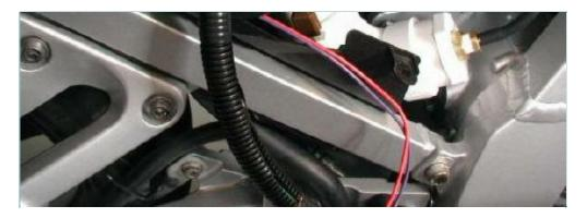
With all the mechanical hardware in place, let's get this thing wired up and get ready to cruise! Start with the wire harness that connects to the servomotor. We can improve on the configuration of the harness by routing some wires and rebundling the harness. Take the Red and Purple wires and place about the last 6 inches near the brown plug underneath the servo.
