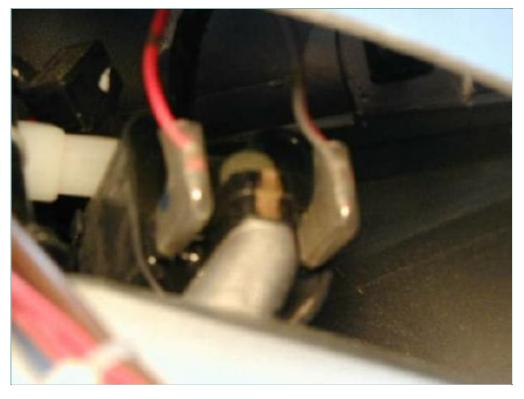
Fasten the Female T-Tap included in the kit to the wire on the coil that is Gray with red markers (the wire on the right) and plugin the Blue wire. This will provide your Tach signal.
