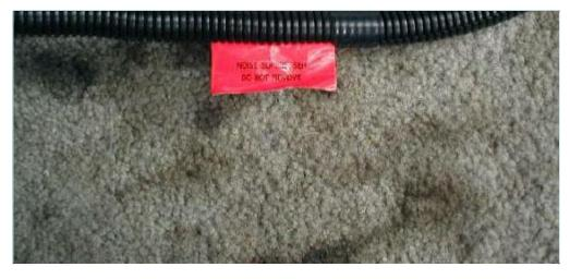
Leave the red label that says "Noise Suppressor - Do Not Remove" sticking out of the harness protector just in case the diode should need to be replaced someday. It will be easier to find.
